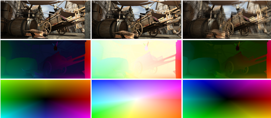
Figure 2.14: Color coding schemes for motion visualization. First row, from left to right : Reference frame, second frame, overlaid frames. Second and third row, from left to right : Flow fields and corresponding color-scheme of Bruhn [40], Middlebury [23], and KITTI [65].
