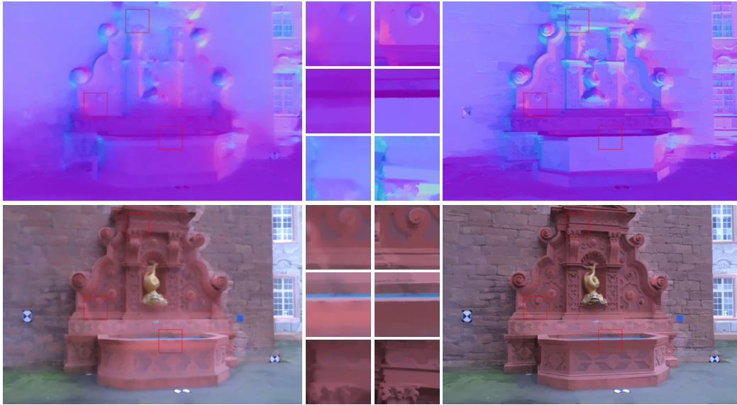
Figure 3.11: Real-world Fountain data set [161]. Top to bottom : Computed illumination direction and computed albedo. Left to right : Partially isotropic model [5] and our anisotropic model.
