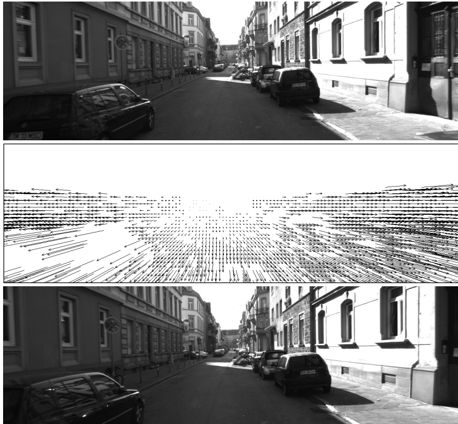
Figure 1.1: Exemplary illustration of the optical flow. Top and Bottom: Two adjacent frames of Sequence 15 of the KITTI 2012 training data set [52]. Center: Vector plot of the 2-D displacement field.
