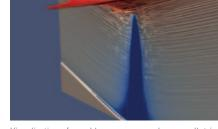
Visualization of a sudden pressure peak on a wall, triggered by the pressure wave of a collapsing bubble.
