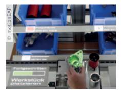
Working station that uses motionEAP technology to display projected assembling feedback as a work assistance.
