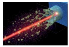
Particle cloud caused by a laser ablation.
